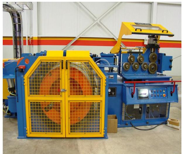
**Figure 3:** Optional Inline Single Drawing Block
