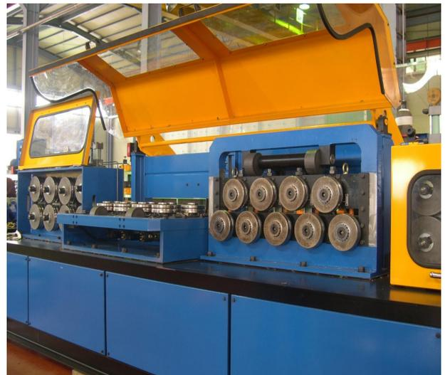
**Figure 2:** Vertical & horizontal straighteners between pinch rolls
