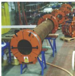
In recent years the name Radyne has gained recognition as a solutions provider to producers of Oil and Gas pipe throughout the world. Radyne is a brand known for provision of high levels of technical expertise and process knowledge on applications calling for onshore line pipe induction heating, prior to surface coating.
